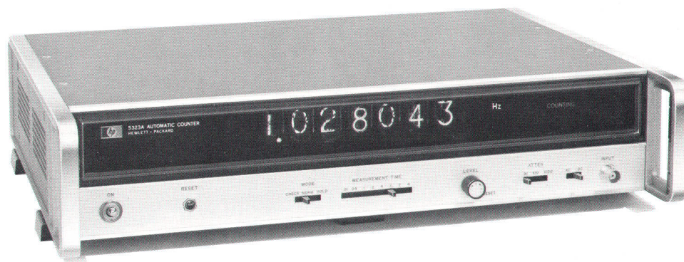
Fig. 1. Model 5323A Automatic Counter measures frequencies by measuring and inverting the period of the input signal. It's completely automatic — the only function control is for selecting the measurement time, which can have non-decade or even (using an external gate) unknown values. Resolution is 7 digits maximum for any frequency, 0.125 Hz to 20 MHz.
